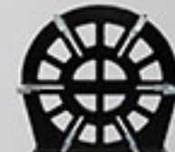
Clamps for welding flange stub
