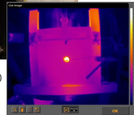
Grit-flame test on 4mm H1030 砂石火烧测试@4.0mm H1030
