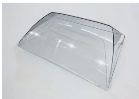
Molded product incorporating recycled PC resin produced using solvent-based technology.
