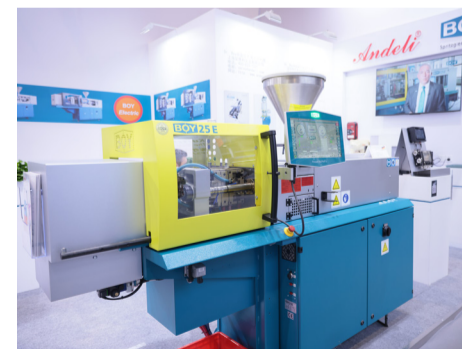
At CHINAPLAS 2026, BOY 25 E produces a threaded rod for dosing an insulin cartridge.
