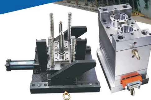
3-5 gallon preform mould
