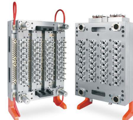
32-cavity Hot-runner Preform Mould
