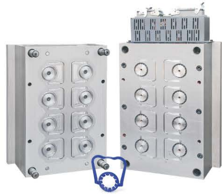
8-cavity Hot-runner Handle Mould
