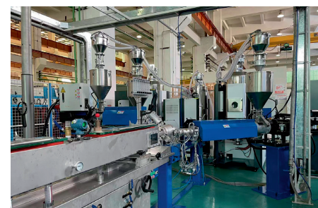
Dekuma's automobile pipeline extrusion line.
