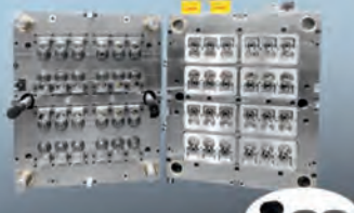
24cav D45 Cosmetic Tube Flip top cap mould 24腔 D45软管翻盖来旋牙模具
