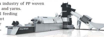
The Repro-Flex is a highly efficient one-step plastic recycling machine for reprocessing different materials.
