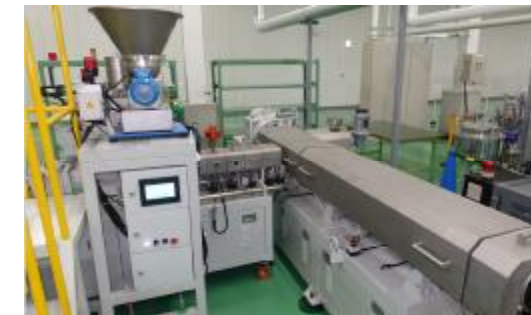
CFE15 /25 双阶发泡实验设备，最高系统压力可达100Mpa CFE15/25 two-stage lab foaming equipment, the maximum system pressure can reach 100Mpa
