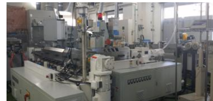
CFE25 /50 双阶发泡实验设备，各种切粒方式可切换 CFE15/25 Two-stage foaming experiment equipment, various cutting methods can be switched
