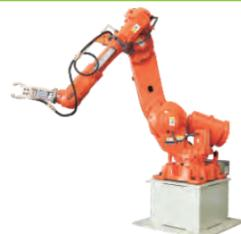
The system can handle parts with a maximum weight of 210kg and biscuit diameter within Φ170. Repeatability is up to 0.02mm.
