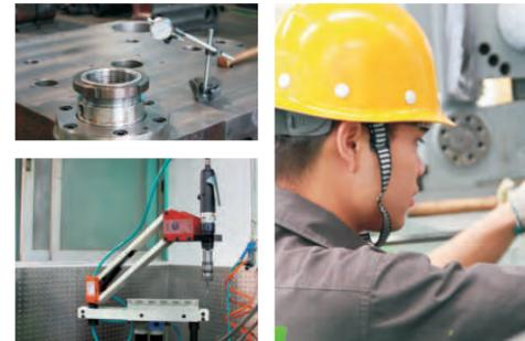
The use of imported pneumatic and electric tools as well as semi-automatic and fully-automatic professional devices in key processes improves the quality and efficiency of assembly.
