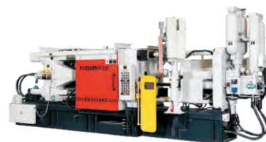
Real-time control technology is also called servo valve control system. Receiving the signal, the control system immediately controls and adjusts the servo valve according to the feedback from the injection process and the signals from the injection position sensor, so fully real-time closed-loop control can be realized.
