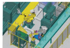
Working with the 6-axis industrial robot, the system features flexible motions, accurate positioning and quick change. It can complete part removal, detecting, cooling, trimming, engraving, marking, transporting, palletizing and other processes automatically.
