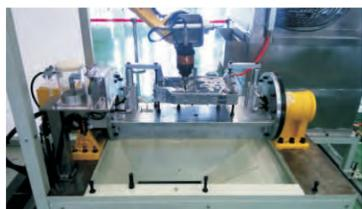
Tungsten steel milling cutter, imported grinding head, functions of tool condition check and spraying, spindle vibration accuracy of 1 μm and removal of burrs with thickness up to 0.2mm
