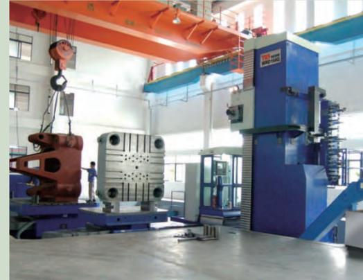
Japan Toshiba MPC-3680EII Gantry Type Five-sided Machining Center
