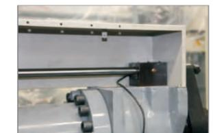
Non-contact injection stroke sensor improves reliability.
