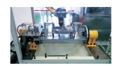
Tungsten steel milling cutter, imported grinding head, functions of tool condition check and spraying, spindle vibration accuracy of 1 um and removal of burrs with thickness up to 0.2mm
