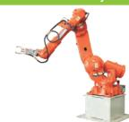
The system can handle parts with a maximum weight of 210kg and biscuit diameter within  $\Phi$ 170. Repeatability is up to 0.02mm.
