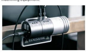
The Machine Tool Precision Detector: XL 80 laser interferometer introduced from Renishaw in UK Main specifications
