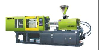
The advanced servo pump technology that SM series adopts can save 20%-80% power compared with traditional injection molding machine, which has the similar effect with the full electric ones. With fast response of servo pump and closed-loop control, the injection molding machine has extremely high repeatability. SM series is available for production with different accuracy requirements.
